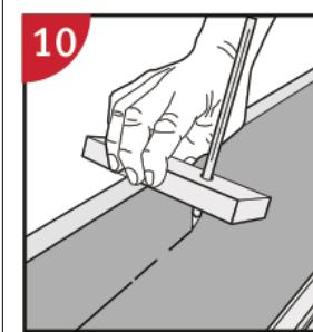
Last row (and perhaps also first row): Always keep a minimum width of 2". Place a spacer to the wall before measuring. Mark the plank along the wall. Cut the planks lengthwise including the flexible tongues and install.
