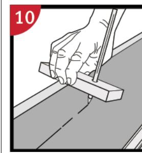
Last row (and perhaps also first row): Always keep a minimum width of 2". Place a spacer to the wall before measuring. Mark the plank along the wall. Cut the planks lengthwise including the flexible tongues and install.
